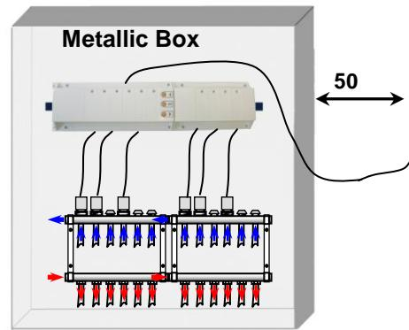
\* For maximum radio sensibility, the active antenna must be placed at a minimum of 0.50 cm of any metallic surfaces (Electrical Box) or vertical metallic pipes.
